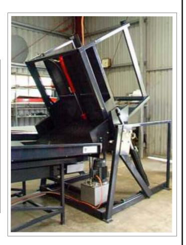
The fruit holding bin is placed into the lifting frame by forklift or pallet jack, the operator then uses a lever to raise the bin to a satisfactory position where a hand operated gate, which is adjusted prior to lifting, helps to regulate the flow of fruit.
