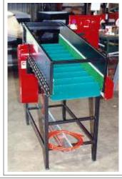
**KW** Automation Brush Polishers come in many configurations to cater to the many varying needs of growers.
