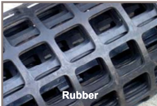
Two 1200mm screens – three grades – up to 20tph
