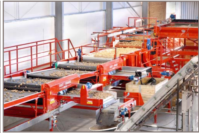
Three 900mm screens – four grades – up to 15tph
