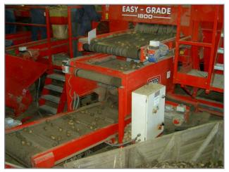
Can be supplied with a horizontal conveyor for crop Can be specifically designed into a grading system
