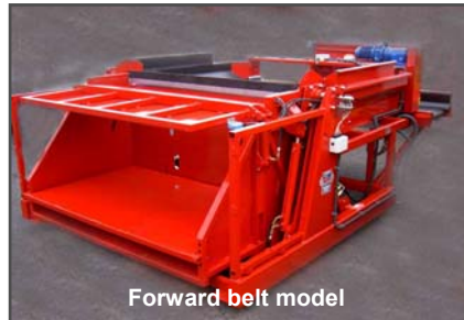
Forward belt model with cross belt
