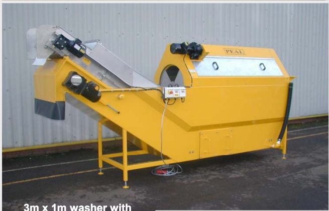
3m x 1m washer with scraper chain
